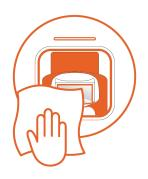
Moisten the cloth or wipe with a suitable amount of rubbing alcohol and gently clean the surface of the fingerprint sensor.
