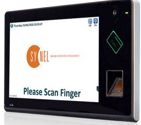
Synel's Synergy Home is an easy to use data capture device delivering enhanced flexibility by combining a high accuracy optical biometric reader for fingerprint based employee logging and the Android based touch screen technology that allows 'self-service' for activity such as logging in and out, requesting absences, checking schedules and much more.
